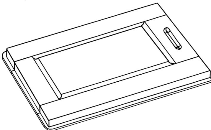
Unless the timber in the lid is quarter sawn and stable, there is a strong possibility of warping, especially with changing humidity. This may result in the lid jamming. The framed panel method can be done on a router table, so it lends itself to the rest of the box making project already described in 'Box making plans'.
