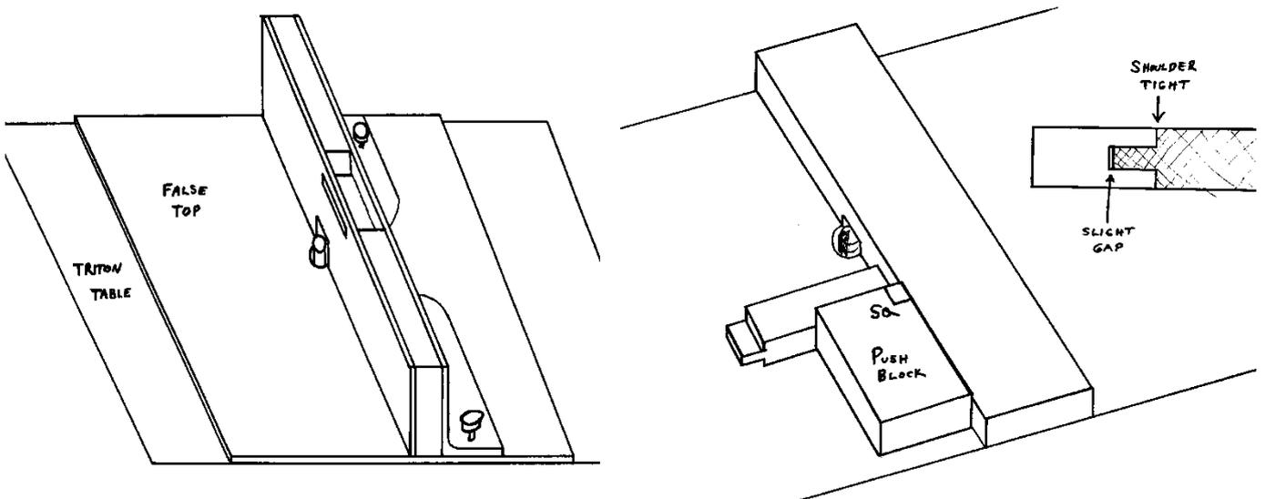
Using a trial piece of wood, run it over the cutter and then turn it upside down and repeat the cut on the other side. Check the fit in the side frame. We want it to be a slightly firm fit, but not tight and hard to assemble. Also check the length of the tenon.
