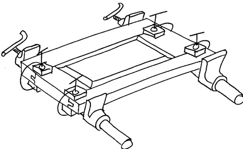
Notice that with this method of construction, both the top and bottom surfaces of the frame are flush with the top and bottom of the panel. This means that we can sand all surfaces (except the rounded rebate on the panel) after the frame is glued. Sand the rounded rebate now.
