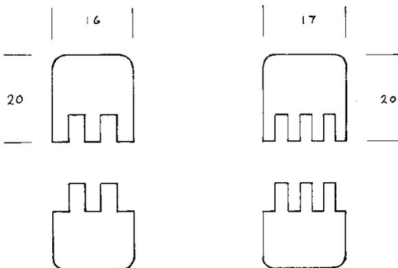
The example in this information sheet describes a hinge for small work—for a box 120mm x 120mm x 60mm. This same hinge can be used on a box 300mm x 250mm x 150mm. There is no reason why the hinge could not be scaled up or down to suit other sized boxes.
