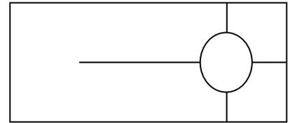
Positioning of the hole is critical for the hinge to work well, so the drilling should be done as slowly as possible. Whilst it is possible to drill the two halves of the hinge together—the drill is more likely to run off. Try it both ways and see which works best for you. If drilling the two halves together, it is necessary to use a 0.25mm spacer (paper or cardboard) to stop the fingers going right home:
