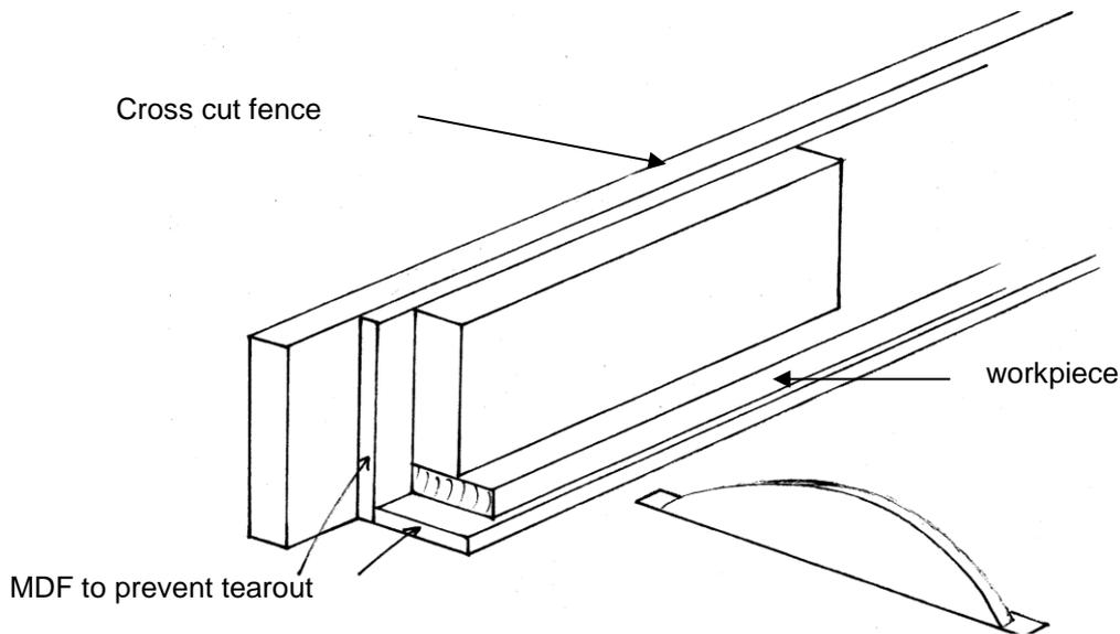
With small work pieces run the work onto the saw, and then stop the saw before you pull the work back off the blade. This is not only safer but also results in cleaner cutting.
