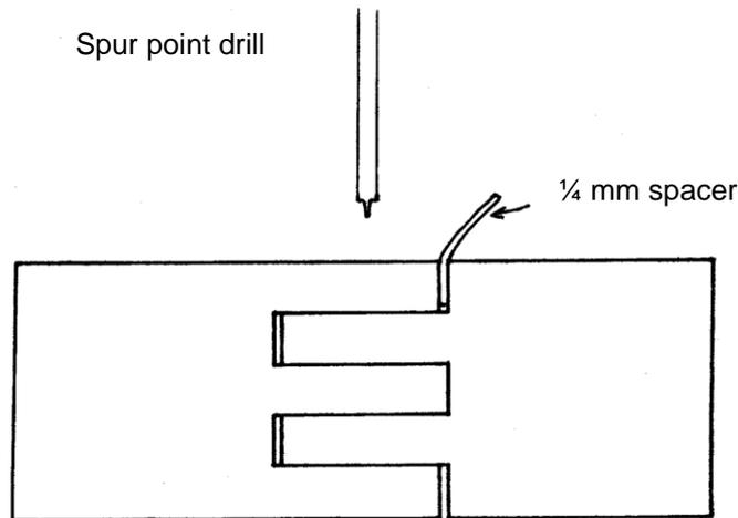
Remember that we allowed 0.25 extra depth when cutting the fingers. This extra depth allows the hinge to swing freely without the ends of the fingers catching on the bottom of the corresponding slot.
