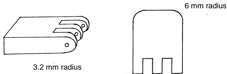
We need to round-over the ends of the fingers (both sides) and also the outside corners of the hinge pieces.
