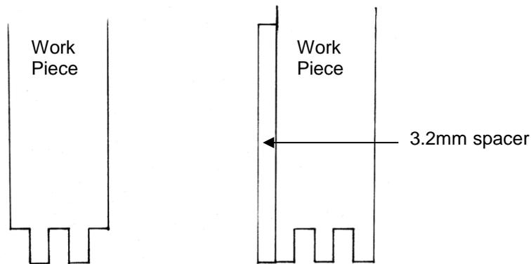
This spacer will offset the second set of finger joints by the finger width, to give us two pieces that will go together with their edges flush.
