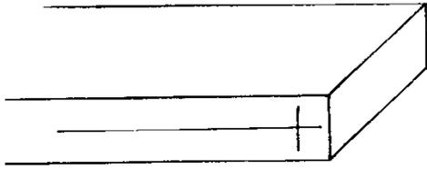
Using a fence and stop block on the drill press, drill a trial hole and check that it is central to the scribe marks both top and bottom:
