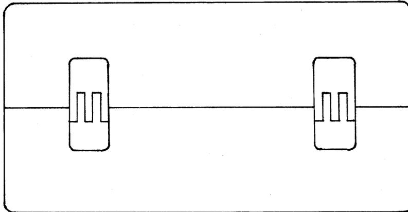
There are two types of wooden hinges, a single action hinge (that is in effect a finger joint with a pin through it) and a double action hinge which has two pins. The advantages of the double action hinge are that it will open out 180°, and you can set it in flush with the back of the box. With the single action hinge, it will only open just past 90°, and it can only be rebated into the box to half its thickness, but it is much simpler to make than the double.
