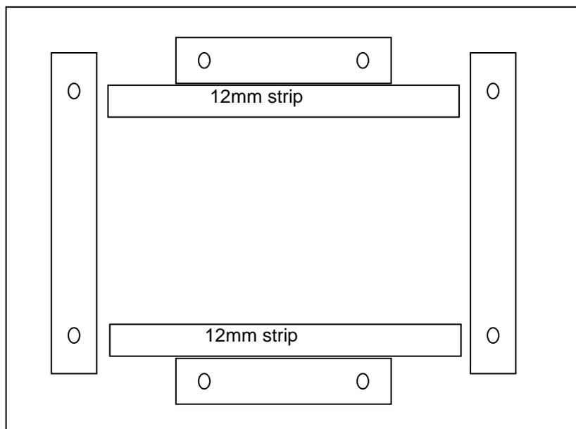
With these strips in place on the jig, increase the depth setting by just over 1.0mm and route the centre portion of the hinge rebate deeper. It is then necessary to clean up the corners for this deeper section with a chisel so we have square corners, rather than round from the cutter. This version of the hinge can now be finished off and fitted in the same manner as described above.
