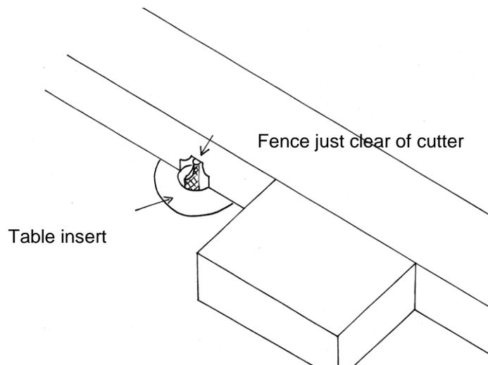
**NOTE:** The drawing above shows the use of a table insert to give support right up to the cutter. The fence is only cut away just enough for the cutter to spin freely. With such a small work piece it needs to be fully supported as it goes past the cutter.
