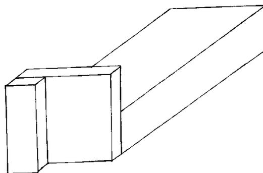
Use a block of 100mm x 50mm hardwood, jointed flat and square before thickening. Cut one end flat and square, and glue and screw a piece of 12mm craftwood to the end as shown. A strip of 12mm craftwood is then glued and screwed to the edge such that it is accurately vertical. Make sure any screws are safely above the cutter.
