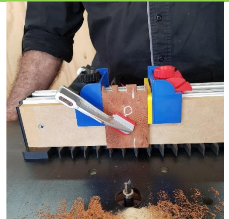
[16] Without moving the jig or the spacers—turn the piece end-on-end. Ensure that the face-side mark is facing out.
