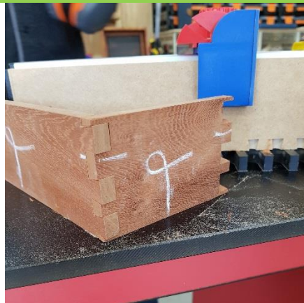
[21] The test joint with a 6mm expanded joint.
