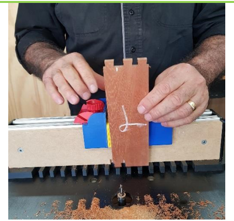
[10] Working from the 'red' stop, cut the half dovetail and expanded dovetail to the chalk mark, then stop.
