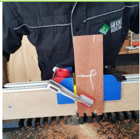
[8] Cut off the overlap to create the expanded joint. Finish cutting the remaining dovetails.
