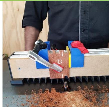
[18] Now change the spacers to the 'black' stop. Do not cut off the overlap.
