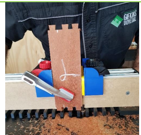
[12] Finish cutting the expanded joint and the remaining dovetails. Repeat this process for the second dovetail side.
