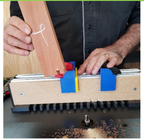
[7] Move the spacers across to the 'red' stop. This will cause an overlap of the last cut joint.
